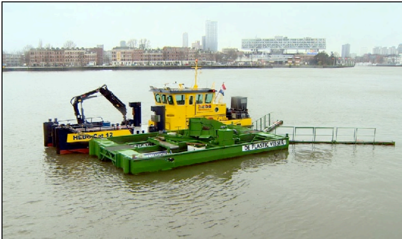
SK international and ISI's Plastic Fisher (above) is a floating platform to retrieve marine litter from rivers. This one's in Nieuwe Maas, Rotterdam, removing plastic before it reaches the North
